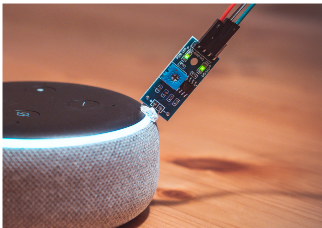
Figure 2: Photoresistor attached to the LED indicator of a smart speaker. The sensitivity of the sensor can be adjusted via a potentiometer. Any activity is recognized and logged.
