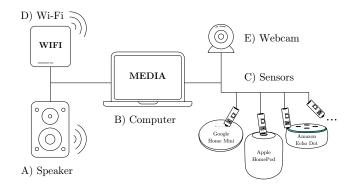
Figure 1: Setup: A loudspeaker (A) is playing media files from a computer (B). The LED activity indicators of a group of smart speakers are monitored using light sensors (C). All speakers are connected to the Internet over Wi-Fi (D). A webcam (E) is used to record a video of each measurement.
