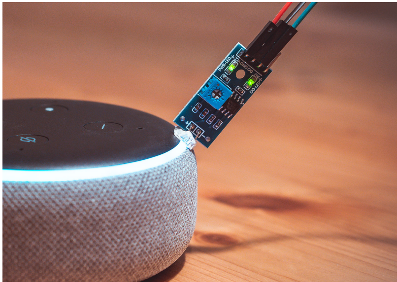
Figure 4.2: Photoresistor attached to the LED indicator of a smart speaker. The sensitivity of the sensor can be adjusted via a potentiometer. Any activity is recognized and logged.
